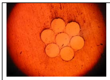
Figure 5-37 The photographs show fibre slicer input (left), fibre slicer pseudo slit with calibration fibres (middle) and slicer pseudo slit (right).
